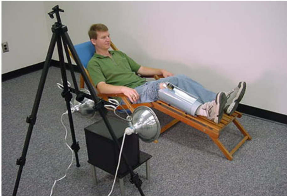
Figure 1 Test setup includes a lawn chair, a custom erythema inducer, a CCD camera and filter-wheel and incandescent lighting.
