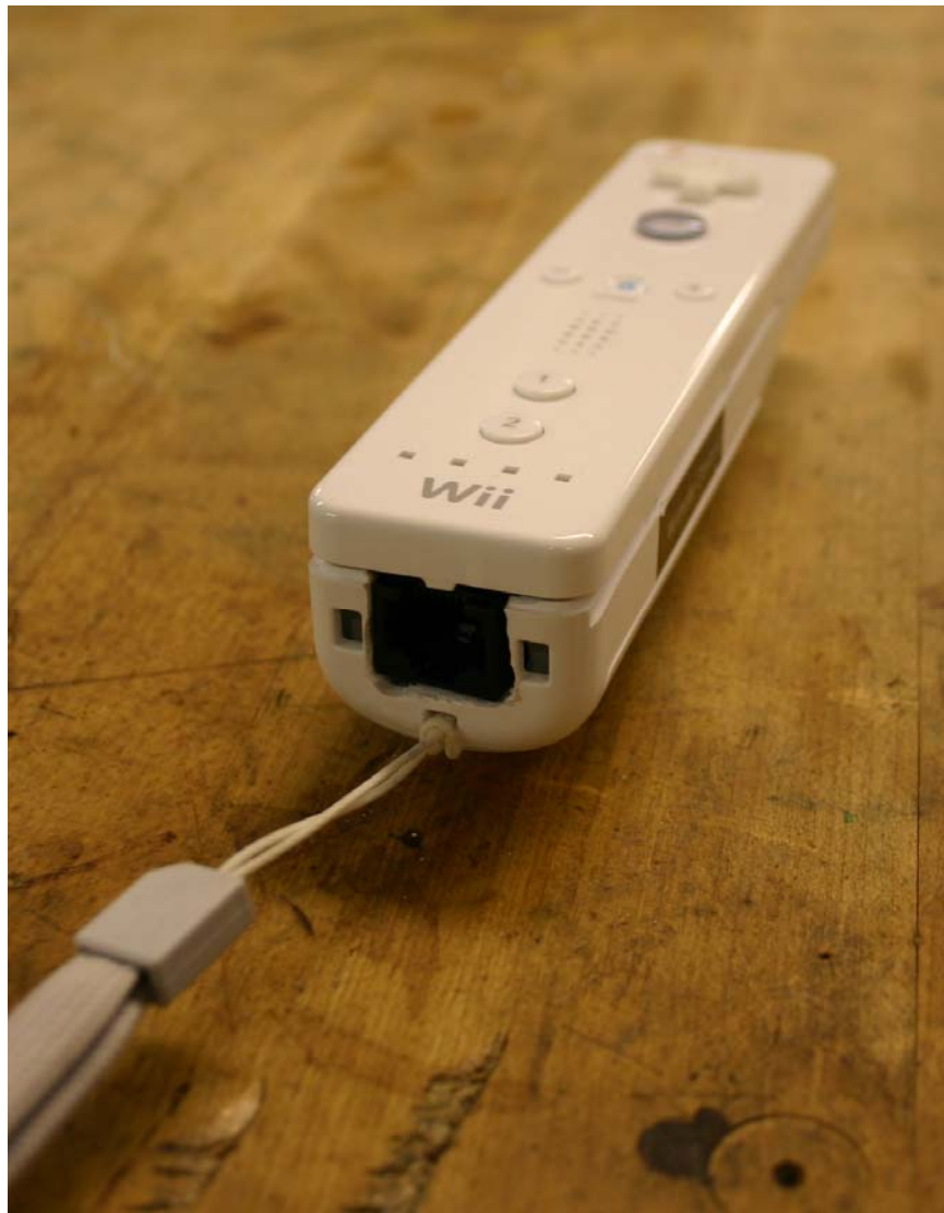
Figure 17: Completed Wiimote with 8P8C Ethernet Port
