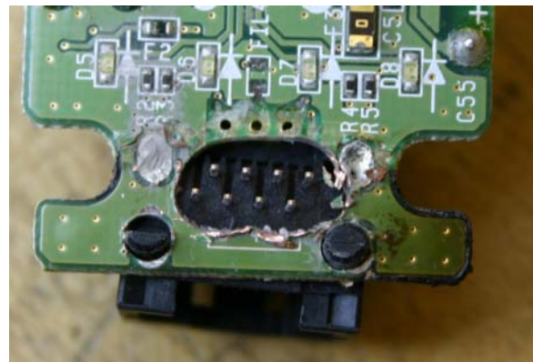
Figure 9: Installation of the 8P8C Female Port.
